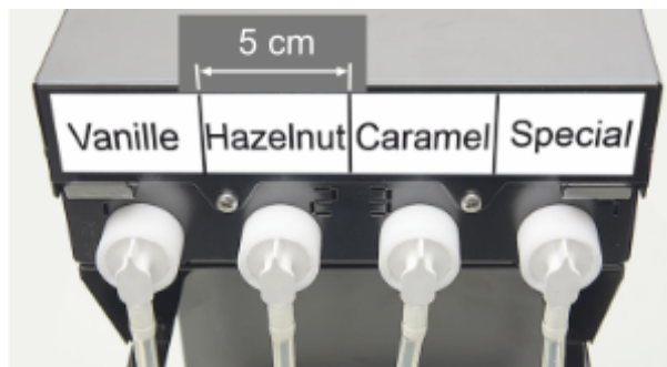
Fig. 48: Labeling example for hose connections from syrup bottle to syrup pump
